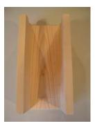
2. Attach the floor. Align the bottom of the floor with the recess guide marks on the sides and back and attach the floor using a good quality weatherproof glue and #7 1 5/8" coated wood screws.
